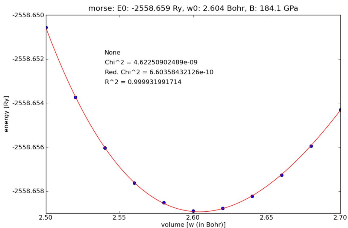
Fig. 1: WS-radius vs. energy curve of fcc CoCrFeMnNi.
