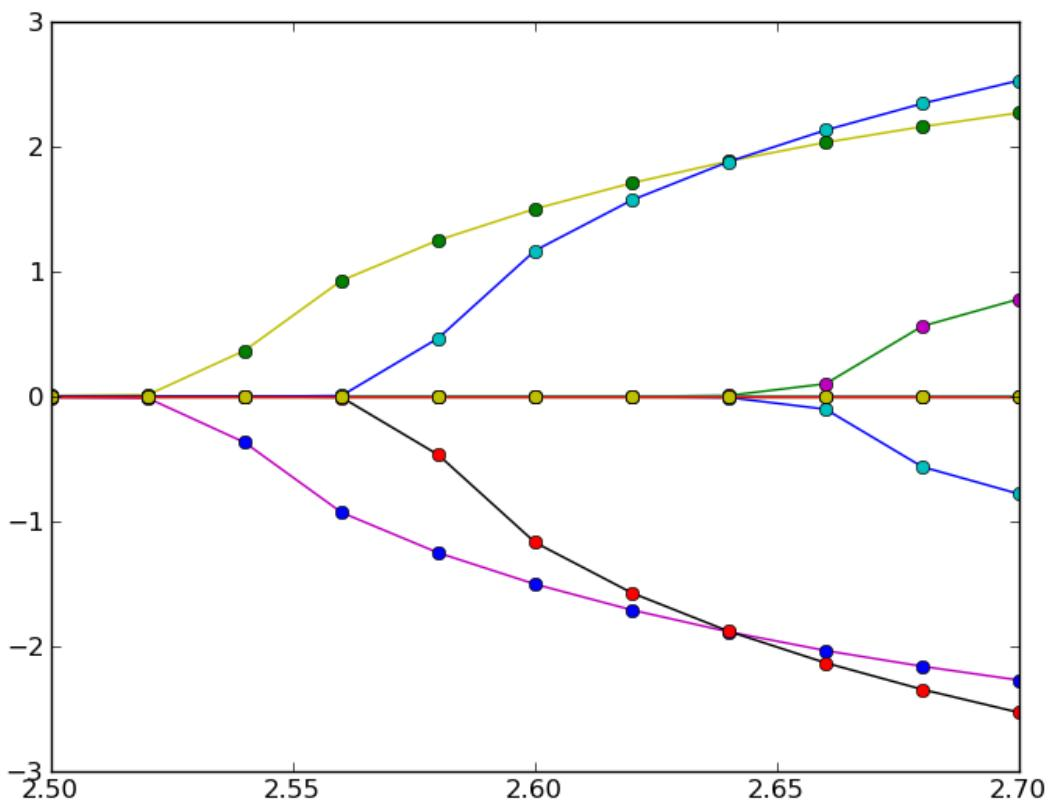
Fig. 2: WS-radius vs. magnetic moments of fcc CoCrFeMnNi.
